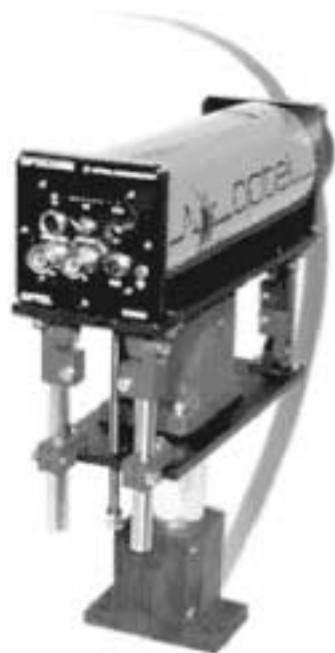
Figure 10-19 Infrared lasers that run at 155 Mbps
